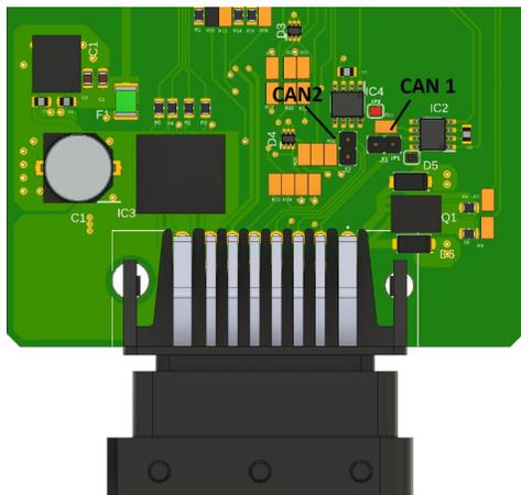
Jumper terminals for CAN bus, left is CAN2 jumper for terminator and right is CAN1.
