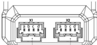
Figure 19: Pin configuration CANbus and power supply
